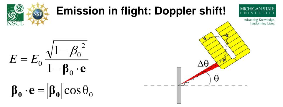
$E_0 \gamma$ -ray energy in the source frame Example: SeGA geometry (NSCL)
