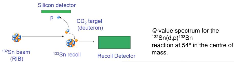
4.77 MeV/u <sup>132</sup>Sn produced and accelerated at HRIBF bombarded a 160µg/cm<sup>2</sup> CD<sub>2</sub> target. Exit-channel proton detection with ORRUBA Si strip detectors under 69-107° polar angles
